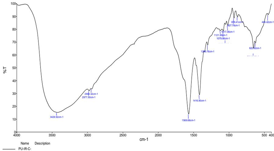
Figure 1. FTIR spectra of HUEP in the range of 400-3500 cm<sup>-1</sup>.
